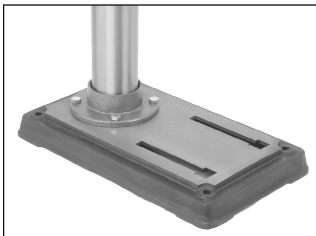
Figure 7. Column secured to base.
